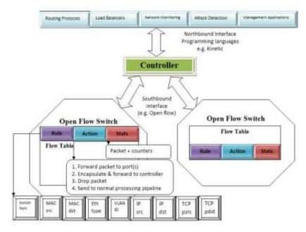
Figure 1 Open Flow-Environment: Flow-based Switching [13] [14] [15]
