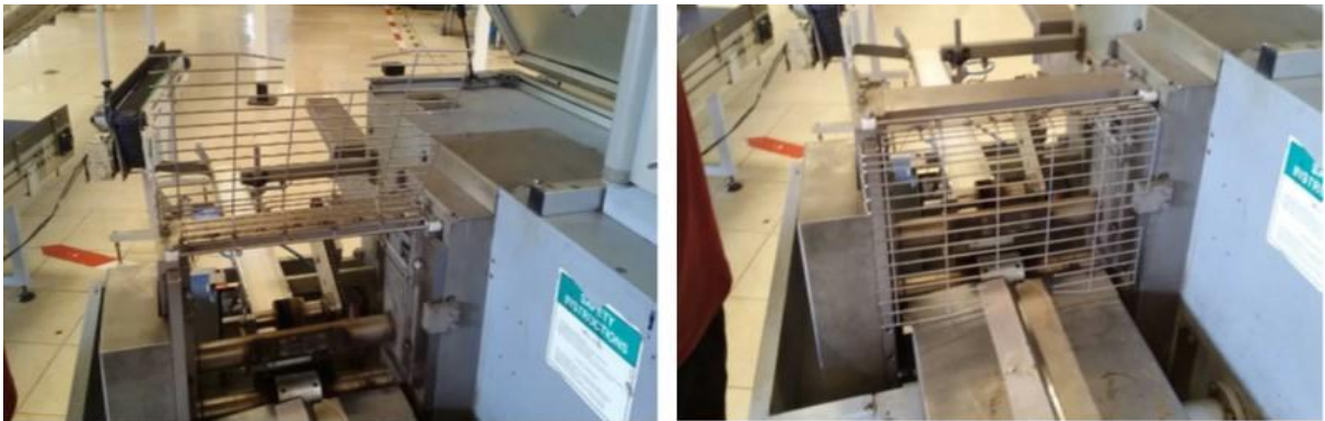
Fig. 10: Adding Safety Frames
