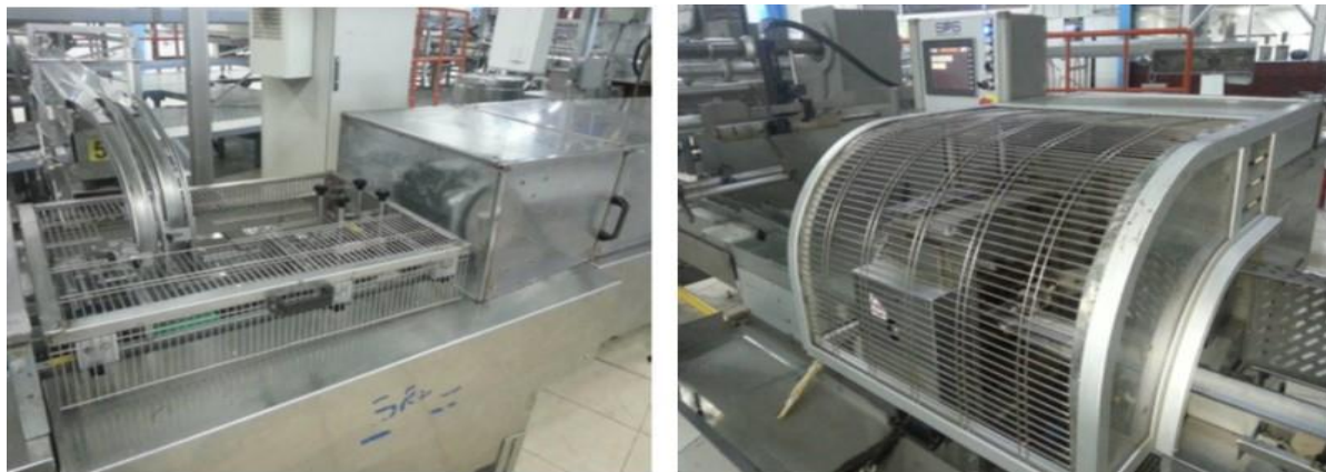
11: Modifications of safety doors
