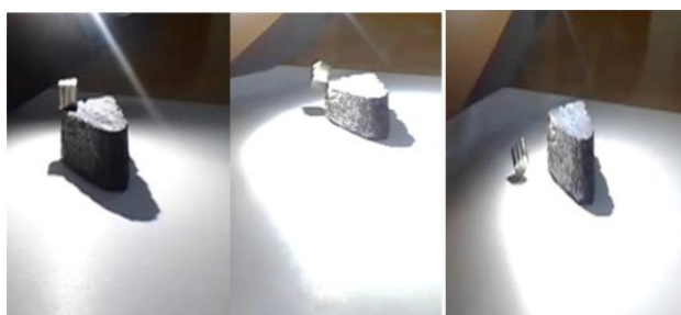
Figure 7: Partial Meissner effect detected at room temperature in the \text{Bi}_{1.7}\text{Pb}_{0.3}\text{Sr}_2\text{Ca}_{n-1}\text{Cu}_n\text{O}_y ( n = 30 ) Bi/Pb-based ceramic cuprate superconductor.
