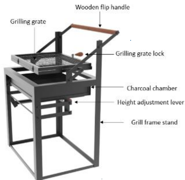
Figure 1. The rotatable fish grill.
