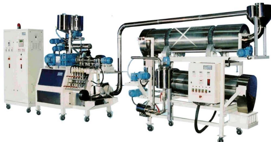
Figure 4: Extrusion system, Model DRX-50, sold by Food Machine Exportation and importation, EIRELI, containing a short barrel extruder, pneumatic transport system to the dryer/flavouring.
