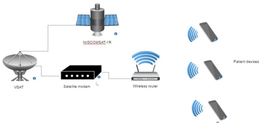
Fig. 2. Connection from the satellite to the community.
