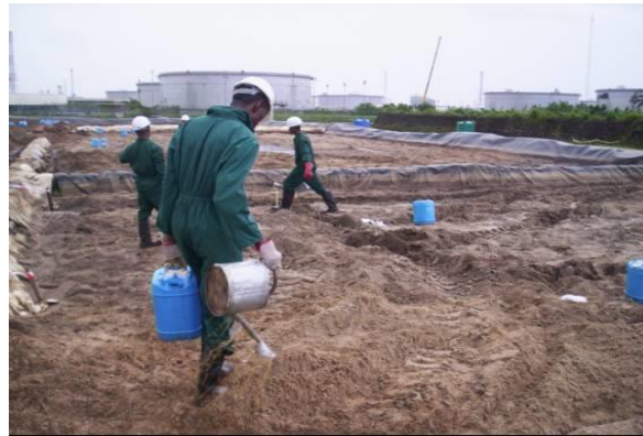
Figure 1: Spiking of the Soil
