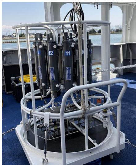
Figure 2: CTD and water-sampling device
