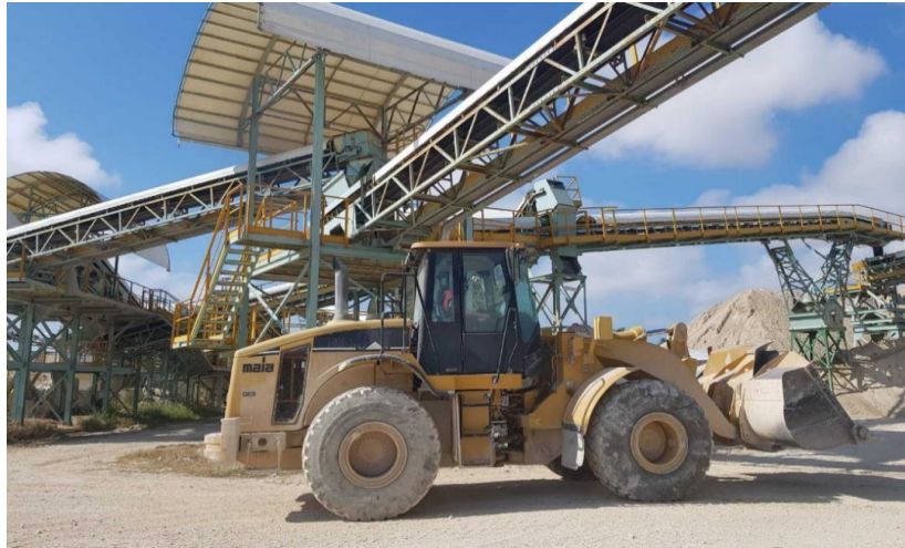
Figure 3: Photograph of a construction waste recovery site showing on-site crushing and sorting, with recycling into road construction materials
