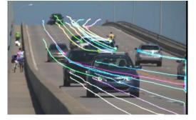
Figure 8. An example of feature-points tracking. (Source: http://docs.opencv.org/master/d7/d8b/tutorial\_py\_lucas\_kanade.html#gsc.tab=0)
