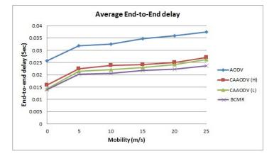
Figure 6. Average End-to-End Delay v/s Node mobility (50 nodes)
