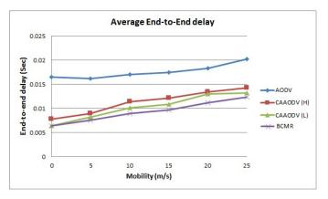
Figure 5. Average End-to-End Delay v/s Node mobility (30 nodes)
