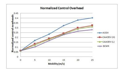
Figure 7. Normalized Control Overhead v/s Node Mobility (30 nodes)
