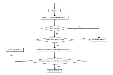
Figure 4. Host's working procedure
